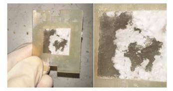
**Figure 2**. Digital image of CaCO<sub>3</sub> precipitated on the membrane.
