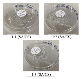
**Figure 1.** Photos of SA/CS spherical gel beads with various ratios of 1:1, 1:2 and 1:3.
