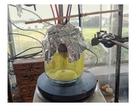
Figure 5. Heterogeneous electrolysis cell reactor
