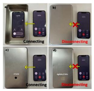
**Figure 7.** The realistic application simulation of EMI shielding for mobile phone communication involves an iron box tested under different conditions: a) open box, b) closed box, c) closed box with a hole, and d) closed box with a hole covered with AgNWs/CNFs paper.
