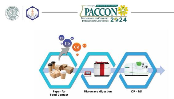
**Figure1.** Schematic diagram of determination of Pb and Cd in food contact paper using microwave digestion followed by ICP-MS.
