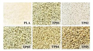
Figure 3. The appearance of bio-plastic pellets with and without oil palm fiber.
