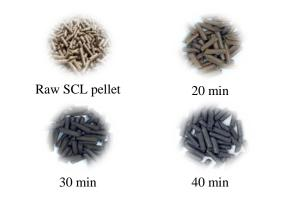
**Figure 6.** Physical appearance of torrefied products at 260 °C at different reaction time
