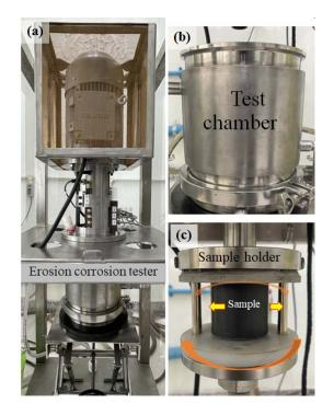
**Figure 2.** (a) erosion corrosion tester; (b) test chamber and (c) sample holder used in this work
