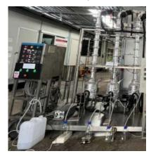
Figure 4. The 3 Columns distillation process.
