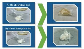
**Figure 4.** An investigation of the fibers' oil and water absorption capacities. The fiber absorbs oil test (A). B) A fiber water absorption test.
