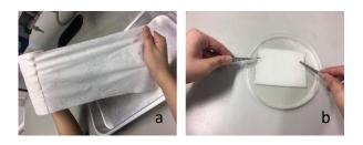
**Figure 5.** Preparation of sanitary napkin by soaking a) bamboo fabric in b) AgNPs solution.
