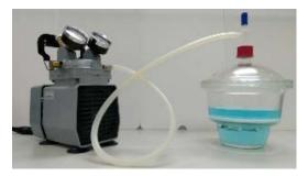
Figure 7. Container closer integrity instrument.
