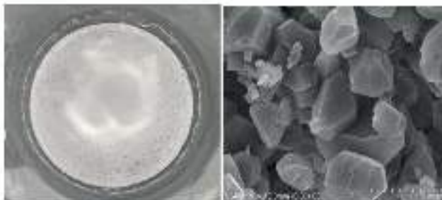
Figure 1. Photograph of amine-captured CO 2 to CaCO 3 by electrodialysis at 0.1 A (left) and SEM image (right)
